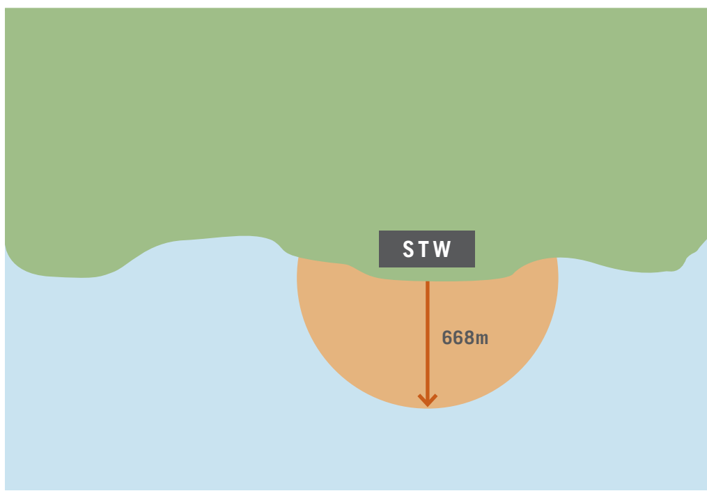
FIGURE A10.4 EXAMPLE OF A BUFFER ZONE BASED ON A SIMPLE DILUTION CALCULATION.
