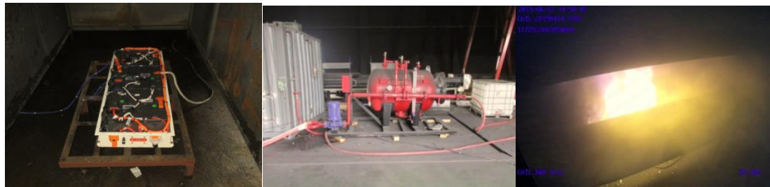
a) battery pack preparation b) fire-extinguishing system preparation c) pack fire
