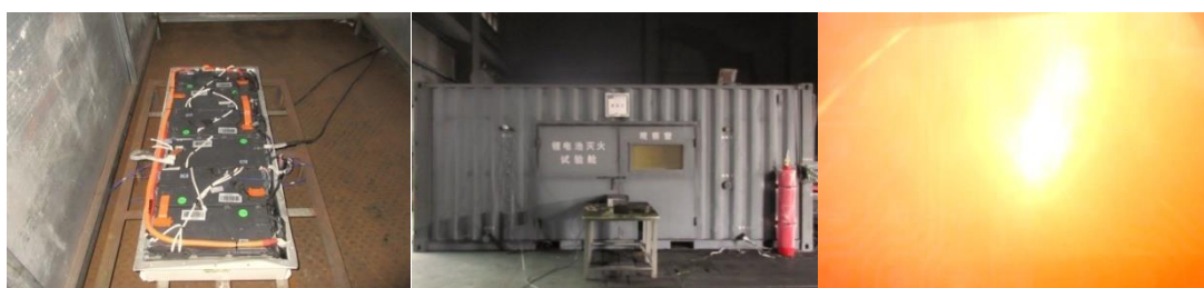
a) battery pack preparation b) fire-extinguishing system preparation c) pack fire
