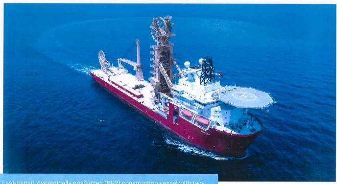
Fast-transit, dynamically positioned (DP2) construction vessel with two 440 ST [400 MT] Offshore Mast Cranes (OMC) and a 625 ST [570 MT] Vertical Lay System (VLS) for installation of flexible pipe and umbilicals.
