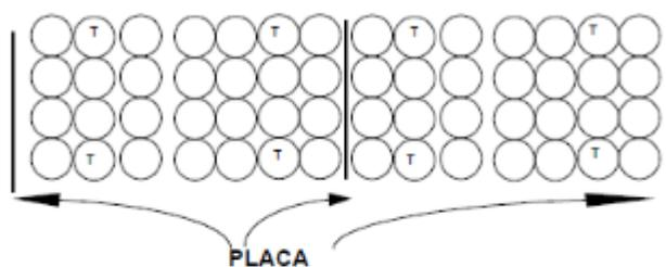
**Colocación de termopares con paredes de placa fría**
