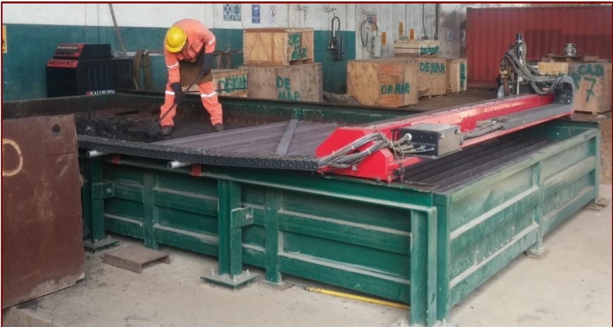
IMAGEN 60: MANTENIMIENTO A PANTÓGRAFO.
