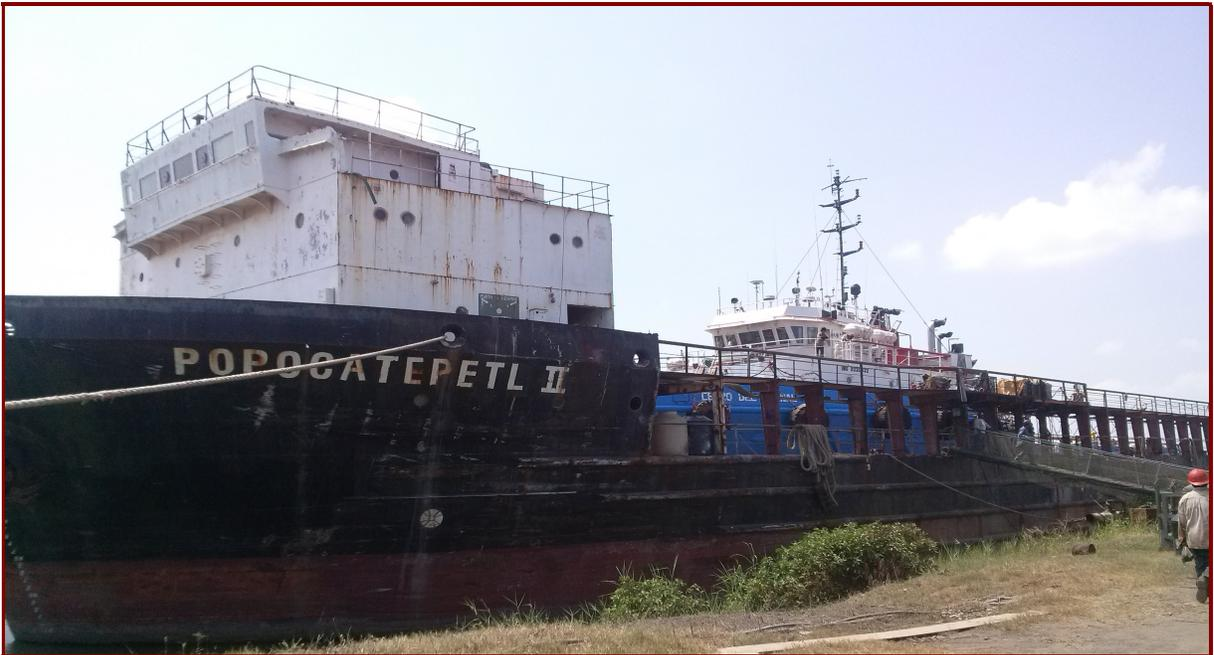
**IMAGEN 50:** BARCO POPOCATÉPETL II CONVERTIDO EN DIQUE FLOTANTE.
