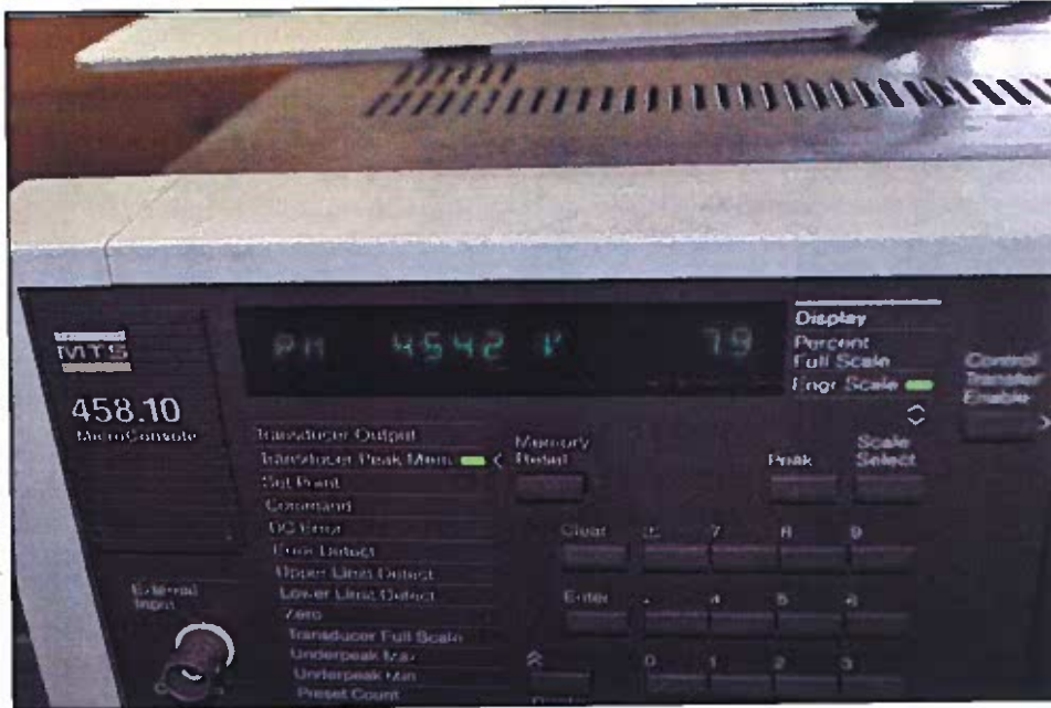
Photo No. 2894-03 MTS signal generator is shown above, which displays peak pressure (at left) and back pressure (right) readings throughout the impulse test.
