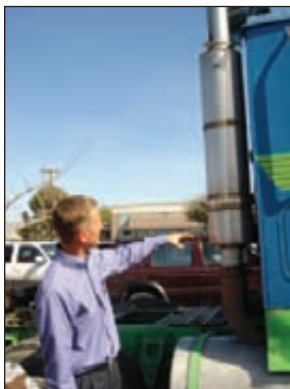
Tim Bradley, Account Manager, Auto Safety House describing the diesel oxidation catalyst pollution control device.
