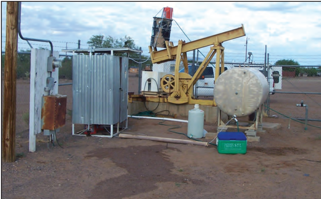
Researchers from Arizona State University test a low-cost treatment system for removing arsenic and nitrates from groundwater on Tohono O'odham lands near Sikul Himatk, Arizona.
