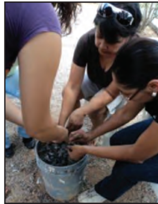
Workshop participants learn how to make fibrous concrete blocks using a mixture of waste paper, cement and sand.
